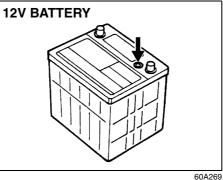
Use only a 12-volt battery to jump start your vehicle. Position the good 12-volt battery close to your vehicle so that the jumper cables will reach both batteries. When using a battery installed on another vehicle, DO NOT LET THE VEHICLES TOUCH. Set the parking brakes fully on both vehicles.  Turn off all vehicle accessories, except those necessary for safety reasons (for example, headlights or hazard lights).
